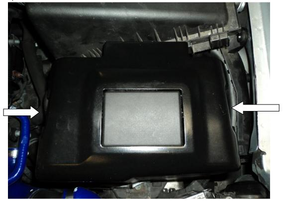
3. Using a 10mm socket and ratchet, undo the two 10mm bolts holding the air box down.
