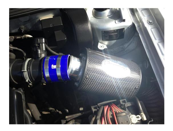
10. Once the pipe is in its position you will need to place the filter onto the silicon pipe along with the hose clamp provided.
