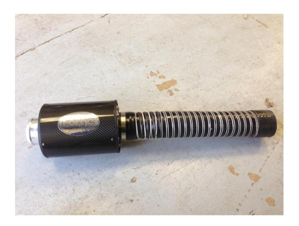
9. Now you will need to fit the filter to the vehicle by pushing the flexible pipe alongside the battery from where the original cold air duct went. It should end up like the picture below sitting under the headlight.
