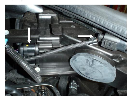
12. Unclip the headlight washer pipe work, undo the two bolts at each end and remove the crash bar. Install the extra capacity crash bar using the bolts just removed and reattach the washer pipe work.
