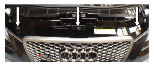
8. Undo the jubilee clips on the intercooler and undo the T30 torx screws on the top and bottom brackets. Keep the top bolts to one side as they are reused on the new intercooler.
