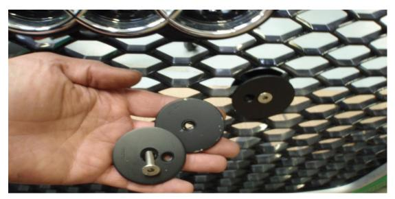
19. Measure between the new number plate fixings and transfer onto the number plate. Drill new holes or move the disc's around until they match up with the existing holes.
