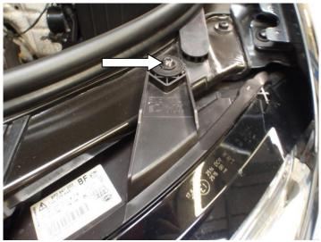
10. Unclip the head light washers and pull off the pipe.
