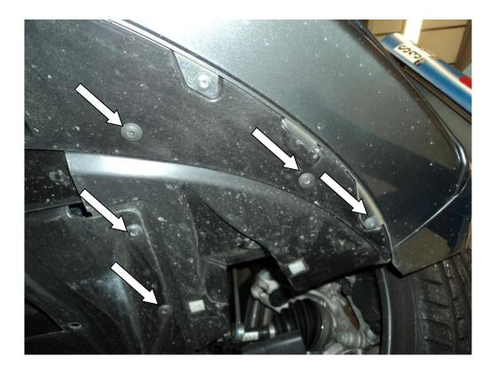
3. Undo the three T30 torx screws at the rear of the under tray then undo the T25 torx screws from the front and sides and remove.
