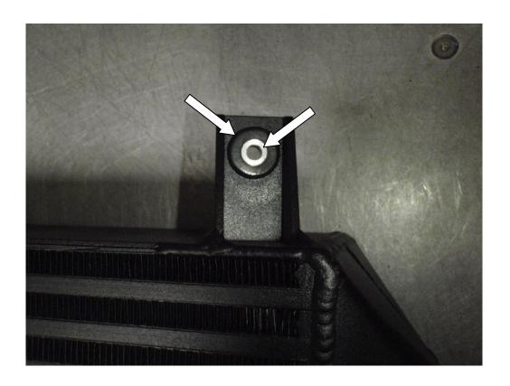
14. Place the uprated intercooler in position, attach the hoses and replace the existing intercooler brackets.
