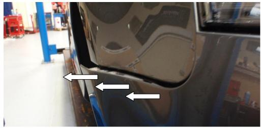
7. Moving to the front of the vehicle, remove the T30 torx screws and remove the bumper.
