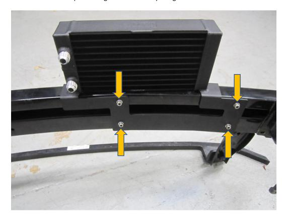
12. As you look at the front of the vehicle, to the top left of the intercooler there is part of the plastic shrouding that needs to be cut down. Cut it as shown in the picture below, measure 29mm up from the bottom and cut straight across with a junior hack saw.
