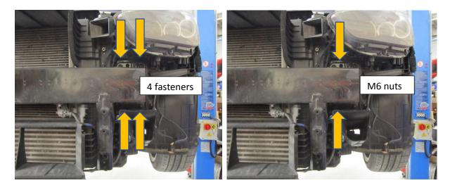
9. With the crash bar removed, place it front side down on the floor or work bench, looking at the crash bar with the lower support at the bottom you will see four predrilled holes to the right hand side. The four holes need to have the diameter increase to 12.5mm use the appropriate drill bit to achieve this.
