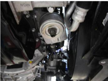
16. Offer up the oil take off plate where the oil filter used to be in the orientation illustrated below, make sure the rubber O ring side is facing towards the engine and secure it in place with the threaded extension supplied. Clean the sealing face for the oil filter, smear a small amount of clean oil on to the sandwich plate O -ring. Use a 26mm extended socket or 26mm spanner to tighten the threaded extension fully, now fit the oil filter onto the threaded extension.
