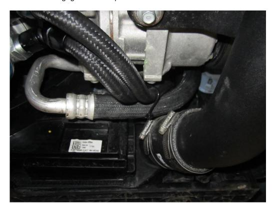
20. Add half a litre of the appropriate grade engine oil to your vehicle to compensate for your new Forge oil cooler. Now start the engine, get it to full running temperature and check for oil leaks, if you do find any leaks; wait for it to cool down and tighten fittings accordingly.
