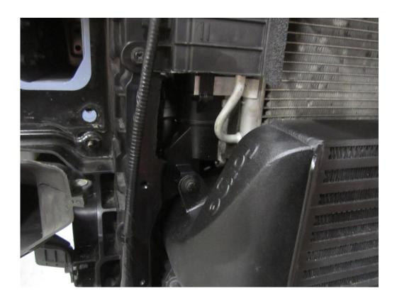
14. Assemble the oil take off plate with the AN fittings and O rings. Attach the 45 degree ends of the oil cooler lines to the AN fitting's as shown in the picture below. Use an adjustable and a 22mm spanner to tighten these fittings, make sure all fittings are tightened firmly.
