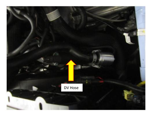
6. Now the Forge DV hose can be fitted using the OE hose clamps, this is the reverse of step 5.
