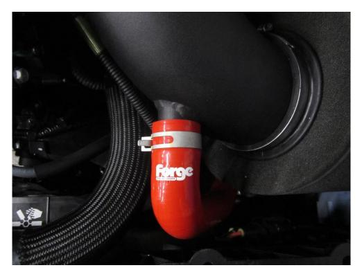
13. Finally, you may need to adjust the position of the air filter, just move into position so that it is not fouling or rubbing and then tighten the hose clamp. The installation of the Forge FMINDK28 is now complete, take your car for a test drive and enjoy.
