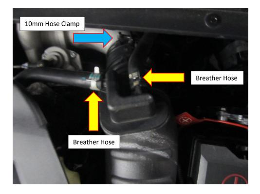
5. With the OE air box and intake pipe removed, you can now access the other end of the DV hose. Once again this is held in place with a spring hose clamp which will need compressing to remove the hose from the vehicle.
