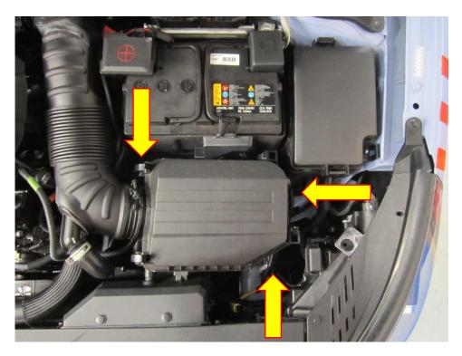
2. Next, the two fasteners that attach the air duct at the front of the air box need to be removed. To do this, gently push the centre of the fastener in with a screwdriver or similar until it loosens, then you will be able to remove the whole fastener from the air duct.
