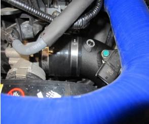
13. Mount the solenoid to the FMBP4 hard pipe using the m6 fastener removed earlier. Use the vac hose supplied with the kit to replace the original hose as this will be too short to re-use. This needs to be used for the diverter valve vac hose also, Cut the vacuum hose to the required length with the use of side cutters then use the provided small cable ties to secure the vac lines in place.
