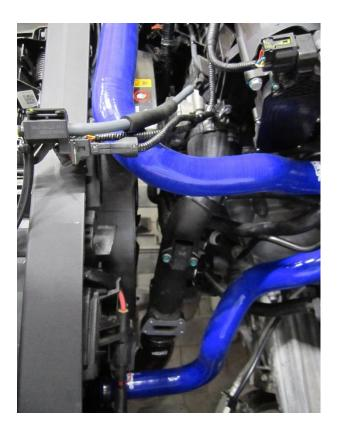
9. Release both hose clamps that attach the boost pipe to the vehicle, there is one which holds the rubber joiner hose to the throttle body and one which holds the 90 degrees joiner hose to the intercooler. Use an 8mm socket and rachet or a flat blade screwdriver to undo both hose clamps. Some clamps may have a cover over the worm drive, this can be removed with plyers.
