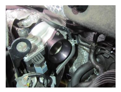
6. With the machined adaptor fitted to the turbo, you will be able to fit the Forge silicone inlet hose. Use the 70-90mm hose clamp provided to secure the inlet hose to the adaptor, fit it loosely at this stage to allow for adjustment.
