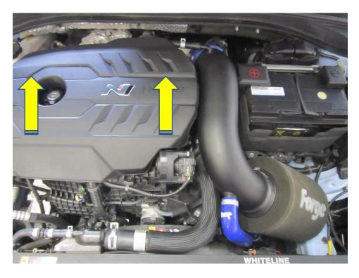
2. Using your hose clamp removal tool or long nose pliers remove the two breather hoses and dump valve recirculation hose from situ.
