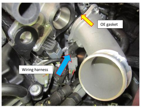
4. Take the Forge Motorsport machined turbo adaptor and offer it up to the OE gasket as shown in the pictures below.
