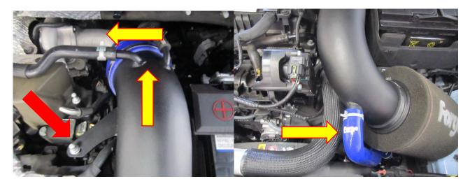
Using a 10mm spanner remove the fastener that holds the intake pipe in situ this is shown in the above picture arrowed in red.
