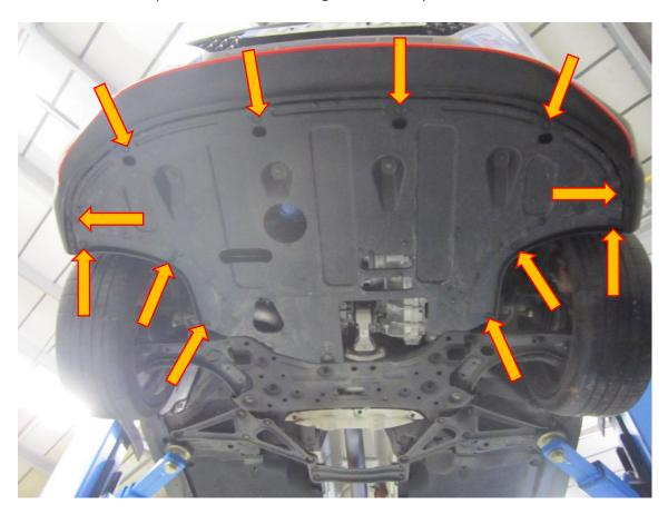
4. Using a 10mm socket and ratchet remove the remaining 7 fasteners left holding the under tray in place.
