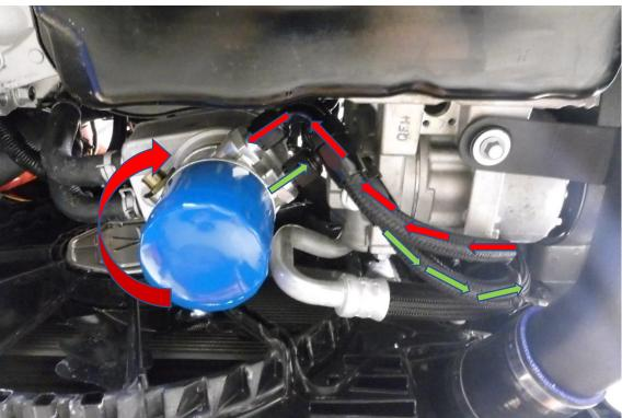
17. Run the hoses as shown in the pictures below, we would suggest you mark one of the hoses with a pen or pencil, so you know which the feed, and which is the return hose. The arrows in green show the feed direction and the red arrows show the return.
