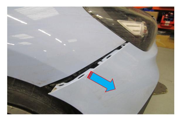
Un-plug both fog lights and parking sensor loom. At this point the bumper can be removed completely from the vehicle.
