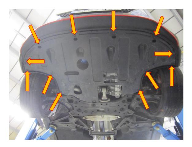
4. Using a 10mm socket and ratchet drive remove the 7x fasteners left holding the belly pan in place and slide it towards the front of the car to remove it.
