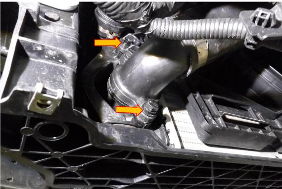
**12**. Using a 10mm socket and ratchet drive remove the 4x M6 fasteners attaching the intercooler to the vehicle. The intercooler can now be removed from the vehicle.
