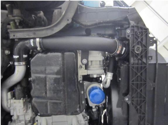
20. Now fit largest hose to the cold side of the intercooler, secure in place using the supplied hose clamps.
