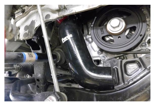
23. Take the hard pipe from the FMINT25 and fit to hose #2043 and using the m6 fasteners removed in step 21 and the supplied M6 nuts, attach the hard pipe in the same location as the original hard pipe. Use the supplied 50-70 hose clamp to secure the larger end of the hose.
