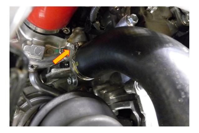
22. Fit the small end of hose #2043 to the turbo, use a 7mm socket and rachet and the supplied 32-50 hose clamp from the kit to secure the hose to the turbo.
