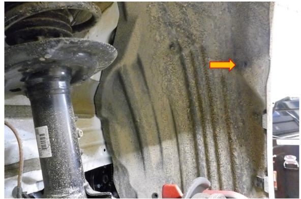
7. Using a 10mm socket and ratchet remove the M6 fastener on both sides of the bumper, the plastic retaining clip also needs to be removed. This simply pushes out of its housing. The bumper will now pull away from the vehicle.
