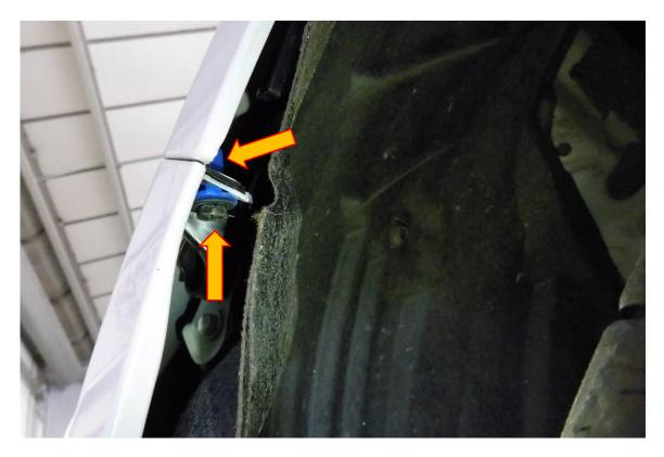
8. Using a plastic trim tool open up the retaing clips to allow the edge of the bumper to come away from the wing. Use some masking tape to avoid marking the paint work. When both sides are free from the wings carefully rest the bumper and unplug both fog light wiring looms.
