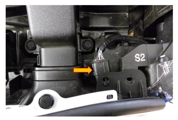
With the vehicle raised from the ground, looking up from below use a 10mm socket and ratchet to remove 10X M6 fasteners at the front of the bumper.
