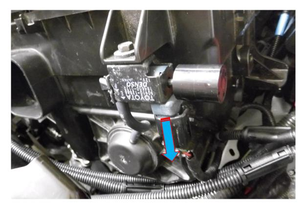
6. Take the Forge Motorsport inlet duct and place it into position. The first picture shows where the fastening points should be located.
