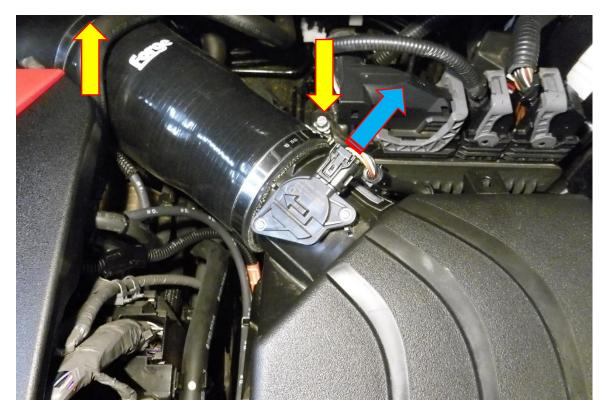
4. Disconnect the vacuum hose from the airbox, and from the airbox pump.
