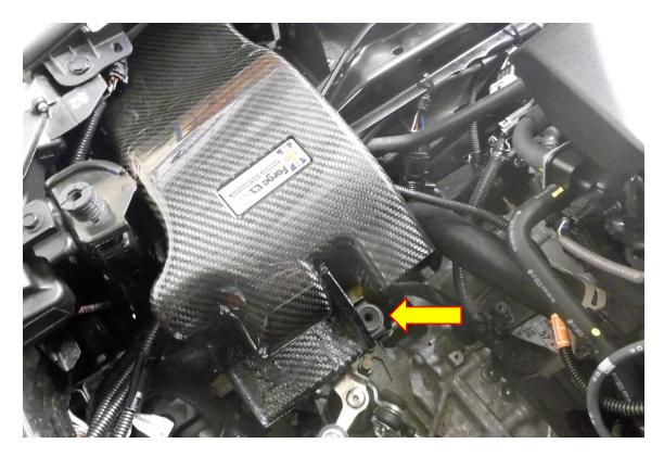
8. When re-installing the airbox re-attach the vacuum pipe to the airbox first.
