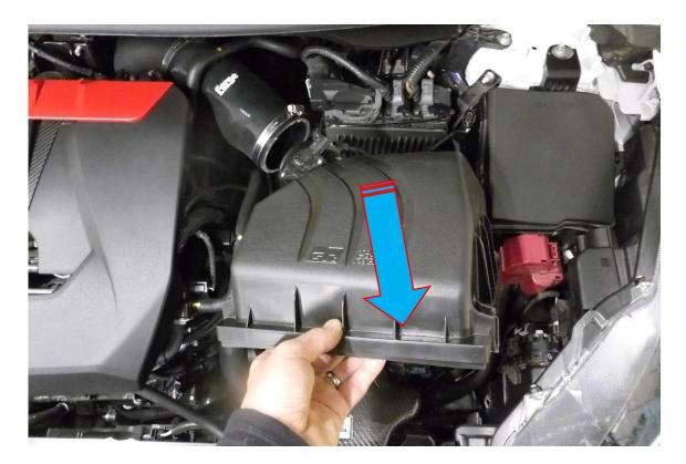
6. Using a 7mm or 10mm socket and ratchet loosen the remaining hose clamp attaching the inlet hose and remove the hose from the vehicle.
