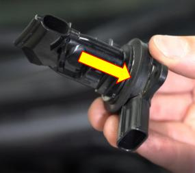
10. Position the MAF sensor into the hole in the airbox as shown in the image below. The arrow will point
