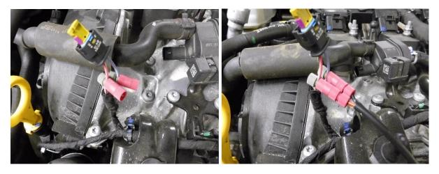
**15**. Cable tie both silicone hoses and the wiring loom to the valve with the vehicles wiring harness running down the side of the engine.
