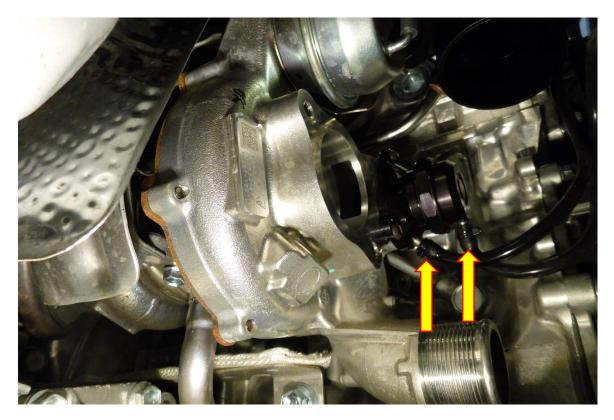
14. Plug the opposite end of the wiring loom from the valve solenoid to the OE valve loom. We have found some vehicles have different plug for the valve, so if you find the loom does not fit your vehicle, we have supplied some wire taps and they are to be fitted as follows.
