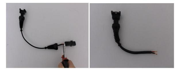
Attach the wire posi taps to the vehicles DV wiring loom first then attach then Forge loom and tighten up to secure the wires. It dosnt mater which way round the loom is connected. (these pictures are library photos from a different vehicle)
