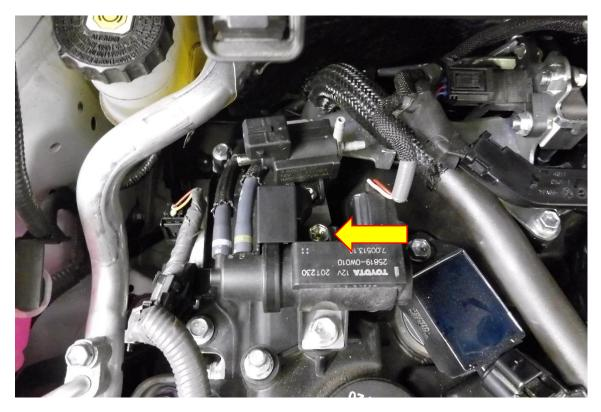
4. Locate the vacuum source which is mounted to the intake pipe. Disconnect the hose on the left side and using some side cutters fit the vacuum T piece and vacuum tube supplied with the FMDV34 kit, fit them as shown in the second picture and run the silicone hose to the solenoid. Secure the hoses with the supplied cable ties.
