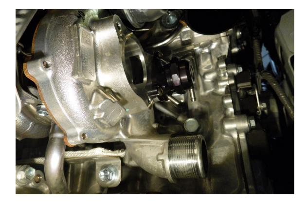
12. Run the new vacuum lines as shown in the diagram below, cut the vacuum tube to length with some side cutters or scissors. Use the supplied cable ties to secure the ends of the vacuum lines to the solenoid and valve then snip off the excess with side cutters.
