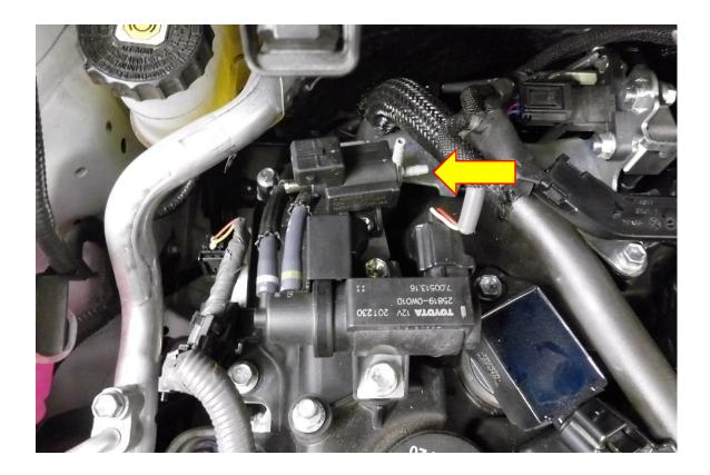
6. Fit the wiring harness to the solenoid, push the plug till you can hear it click into position.
